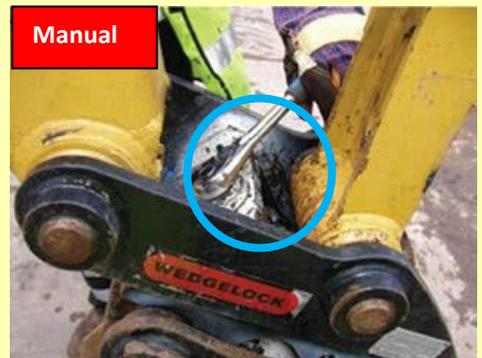
With ratchet operated retaining mechanism
