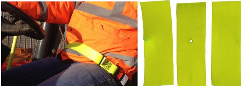
The areas to check are the seatbelt webbing, the buckles/fixings and the retractors. Wear and tear or abuse can affect all these parts. At no point should the retractable seat belt be tampered with to make it a lap belt (adding knots to the webbing).
